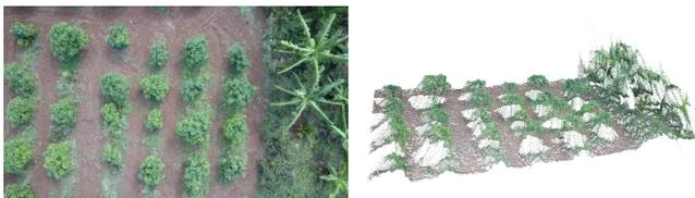
Fig. 10. a) Input Imagery (Left) b) Generated Point Cloud (Right)
